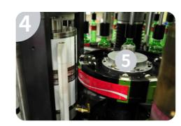
**Labeling Station** The labeling station, which may be adjusted either vertically or horizontally, handles containers in different diameters and labels in different heights.
