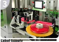
The reel roller, cutting unit, vacuum-grip cylinder and Glue unit are driven by computer-controlled servomotors. Automatic Reel Storage Magazine (Optional)provides continuous 4~6 hours non-stop labelling supply.
